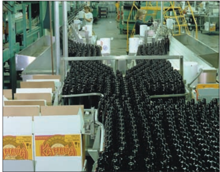
Baldor Washdown Duty Motors provide easy clean up for Hiram Walker's high speed, bottle filling line. The line fills Kahlua bottles at a rate of 300 bottles per minute.
